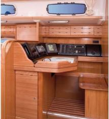
Chart table with large compartment for charts and wrap around console for navigational instruments
