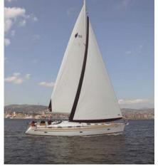
• Double spreader Selden mast, choice of conventional, furling or fully battened mainsail, adjustable pneumatic boom vang and top quality deck hardware
