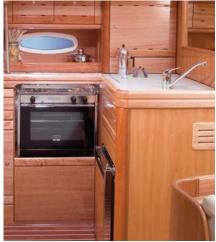
• European style galley with ample counter space and storage lockers, propane stove with oven and front opening 12 Volt refrigeration
